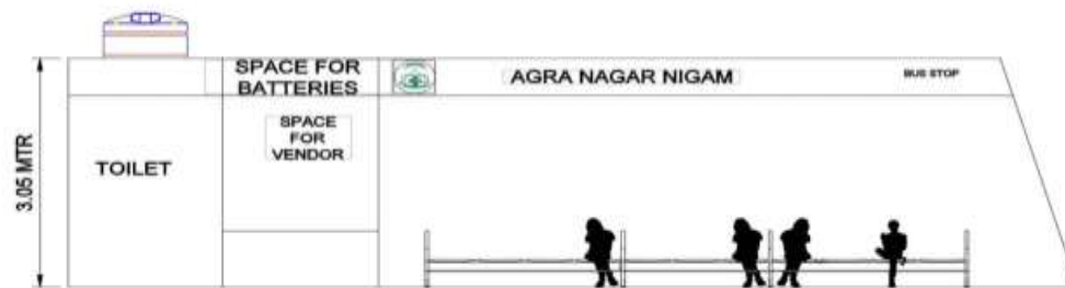
SECTION OF BUS SHELTER
