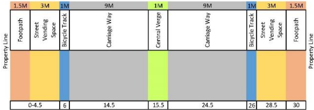
Figure 29 Proposed 36 M wide Road cross section
