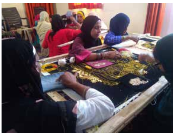
Figure 7: Zardozi artisans working around the 'adda' i.e. the wooden frame, which can accommodate four to six artisans working together. Source: Authors
